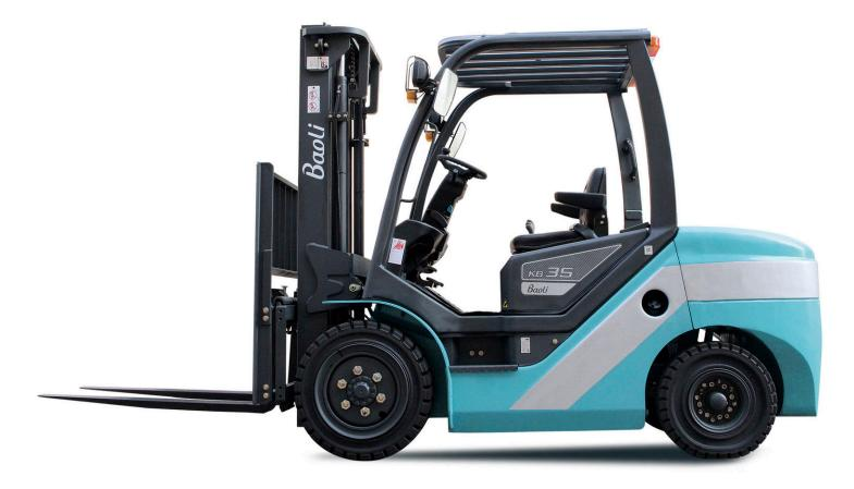
1.5 - 3.5T Internal Combustion Forklift Trucks (Diesel)
